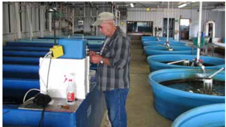
Don Thran stands before a tagging machine that inserts a small wire tag into the snout of the sturgeon.
